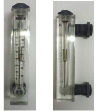
4. Flow Meter (front and side view)
