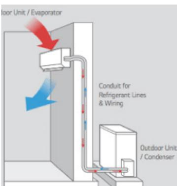
Multi-zone systems are commonly ductless and condition up to eight rooms (zones) from a single outdoor unit. While these systems are often easy to use, in order to achieve ideal redundancy, excessive amounts of equipment and electrical infrastructure is needed
