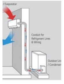
the heat from the air inside the space and transfers it to the condensing unit outside the grow to be rejected.
