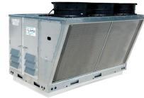
These unit's cooling and heating functions are the same as standalone DX systems, however the dehumidification function is combined into the same unit, so they work in concert. There are two forms of hot gas reheat. There is an on/off type with poor discharge air temperature control (but less expensive) and complex modulating which offers better discharge air control but is more expensive.
