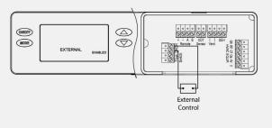
The Model S710 can be controlled with the Model S77 Control (included) or any external control that can provide a dry contact closure. When the Model S77 is used, the User Interface on the dehumidifier **MUST BE** set to "Remote". For all other external controls, the User Interface **MUST BE** set to "External". Refer to the quick start guide or installation manual for instructions on accessing the installer set-up menu.
