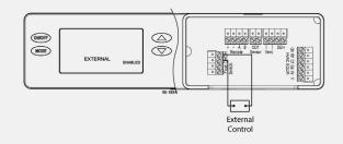
The Model S710V3 can be controlled with the Model S77 Control (included) or any external control that can provide a dry contact closure. When the Model S77 is used, the User Interface on the dehumidifier **MUST BE** set to "Remote". For all other external controls, the User Interface **MUST BE** set to "External". Refer to the quick start guide or installation manual for instructions on accessing the installer set-up menu.
